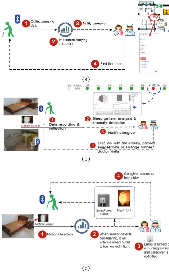
**Fig. 1.** Flowcharts of three scenarios, including (a) straying detection, (b) sleep pattern detection, and (c) night-time bed-leaving detection.
