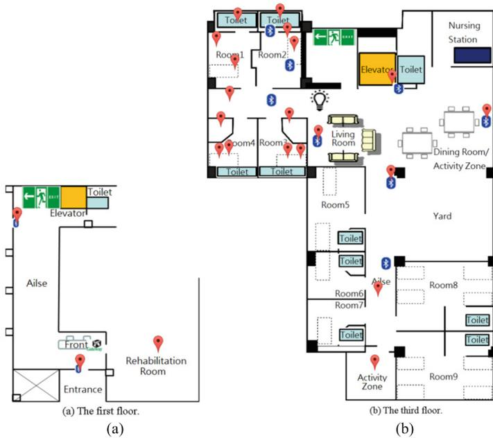
**Fig. 2.** Sensor deployment in (a) the first floor, and (b) the third floor in the caring facility (Color figure online)
