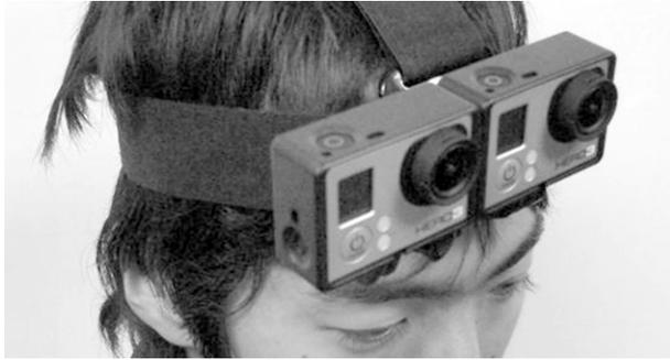
**Fig. 2.** Two cameras mounted on a walker's forehead to capture stereo motion images or 3-D optic flow.
