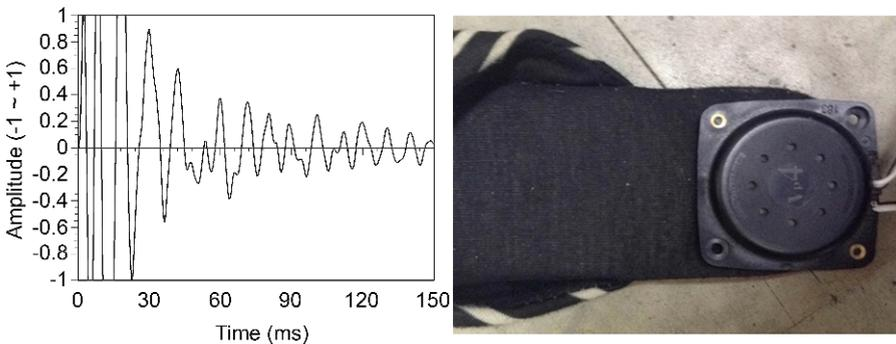
**Fig. 6.** (Left) Vibration profile. (Right) A vibro-transducer attached to a shoe
