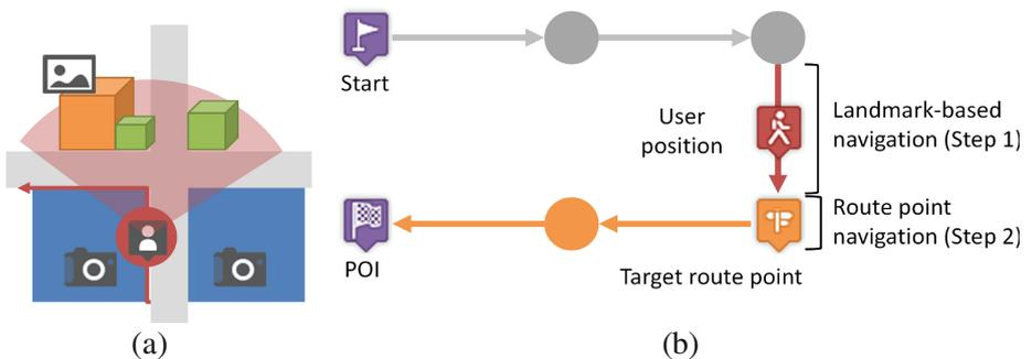
**Fig. 2.** Process of landmark-based pedestrian navigation: (a) landmark and social media selection-based route path and (b) partitioning route path into landmark-based path guide (Step 1) and direction guide to next route point (Step 2). (Color figure online)
