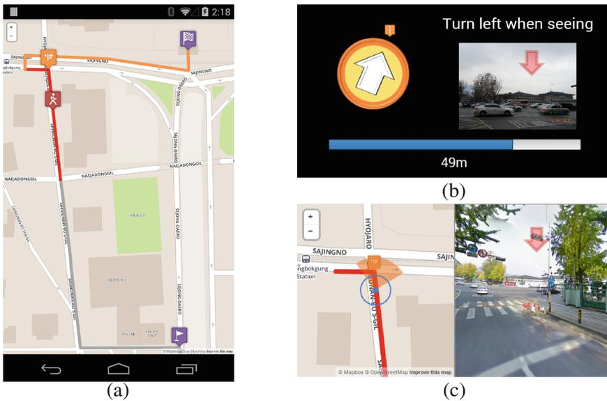
**Fig. 3.** Implementation of pedestrian navigation system: (a) Overall context on hand-held device (Google Nexus smartphone), (b) landmark-based navigation for finding route point on wearable device (Google Glass), and (c) route point navigation for turning to next route point on wearable device. (Color figure online)
