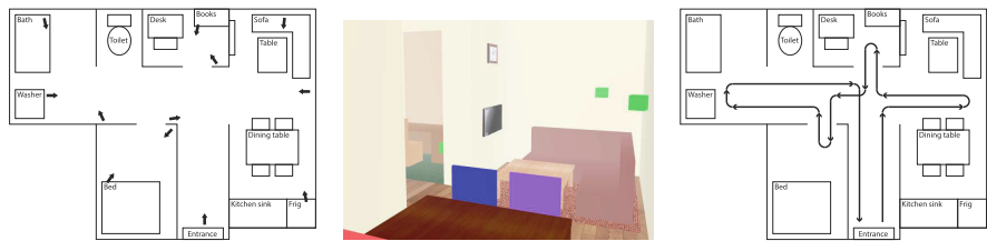
Fig. 2. Design of navigation methods. The pre-defined viewpoints for Click method are shown to the left and they are rendered as green cubes as shown in the screenshot in the center. The pre-defined path for Auto is shown to the right. (Color figure online)
