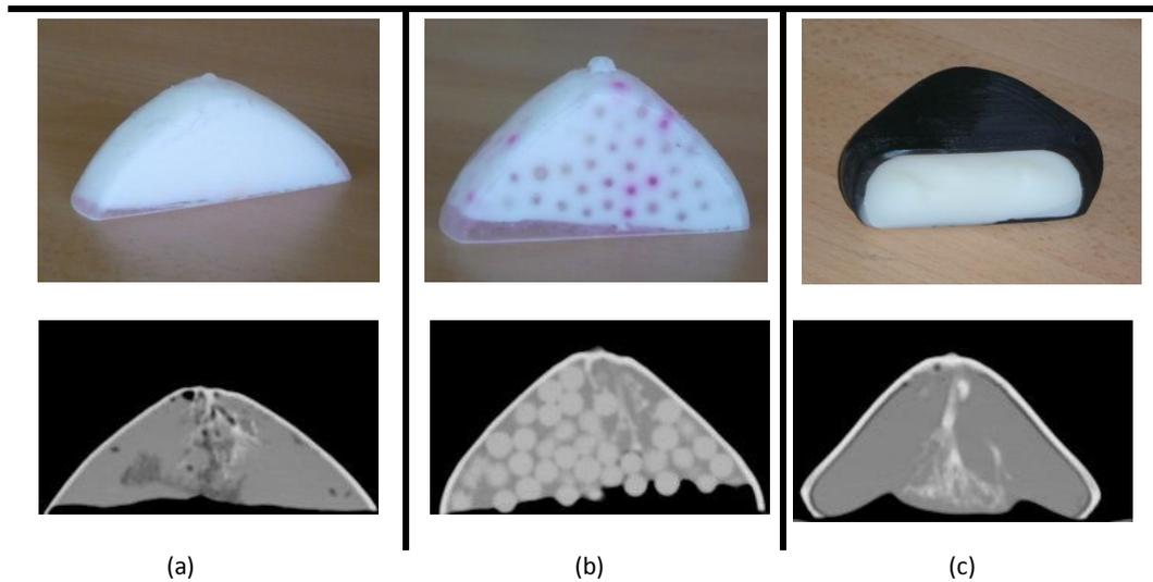
**Fig. 5.** In-house developed breast phantoms (upper row) and their tomograms shown in the second row.
