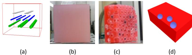
**Fig. 1.** Photographs and sketches of the physical phantoms used in the experimental work: (a) arrangements of the nylon fibers with diameters ranging from 0.08 mm to 0.40 mm; (b) phantom with nylon fibers embedded into a paraffin mixture; (c) water spheres embedded within a paraffin slab.
