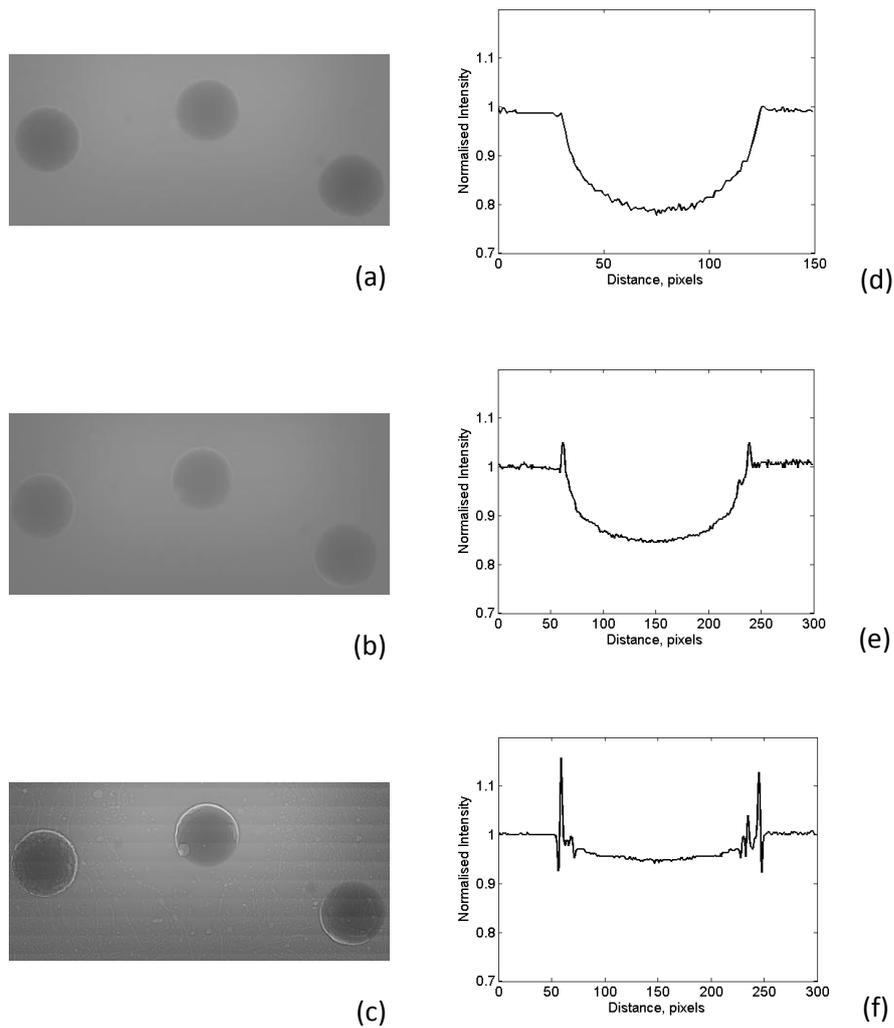
**Fig. 2.** 2D images (a, b, c) and corresponding line profiles (d, e, f) (taken across the middle sphere) of the paraffin slab with the three water-based spheres. The images were acquired with (a) a GE Senographe unit at 28 kV, and (b, c) at the ESRF beamline ID17 at 25 keV.
