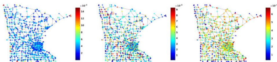
Fig. 2. Sampling probability distribution p_s in different scales derived from “Meyer” wavelet on Minnesota graph. Left: at scale s = 1 , Middle: at scale s = 2 , Right: at scale s = 3 .
