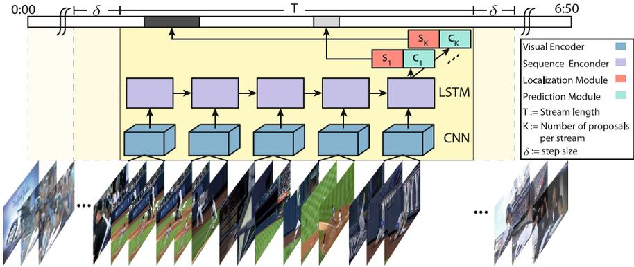
**Fig. 2.** Our Deep Action Proposals (DAPs) architecture effectively encodes a stream of visual observations (of length  $T$  frames) into discriminative states from which it is possible to localize  $K$  proposals  $\{s_i\}_{i=1}^K$  with confidences  $\{c_i\}_{i=1}^K$  inside the stream. We generate several segments where it is possible to find actions along a video sequence by sliding it with step size  $\delta$ .
