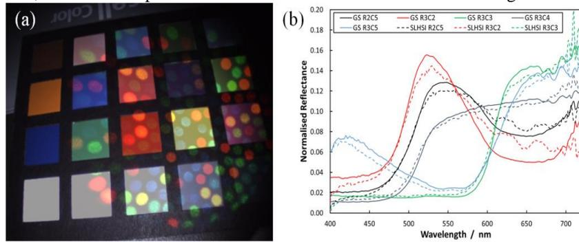
**Fig. 3.** (a) Macbeth colour chart illuminated with SL. (b) Reflectance spectra from selected colour panels of the chart, with  $R$  and  $C$  indicating the row and column, respectively. Data from the hybrid system (SLHSI) are plotted alongside the high resolution spectrometer results (GS).
