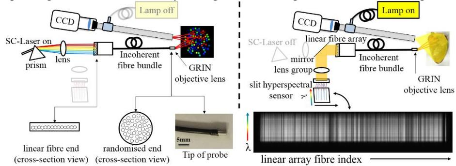
**Fig. 1.** Left: setup in SL mode, and the physical appearance of the miniaturised probe (lower left). Right: setup in HSI mode and the captured spectrograph image (lower right)
