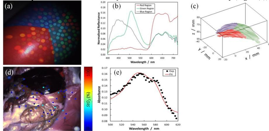
**Fig. 4.** (a) Three-coloured cylindrical target with SL. (b) Mean reflectance spectra for each of the target's regions. (c) 3D reconstruction coloured by RGB values generated from spectra in (b). (d) Murine abdomen with  $StO_2$  overlay. (e) Tissue absorbance spectrum and model fit.
