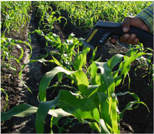
Fig. 2. Canopy temperature measured by infrared thermal imager
