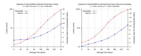
Fig. 7. Performance of linear scaling shmem\_collect64 and recursive doubling shmem\_fcollect64 for variable message sizes on 16 processing elements
