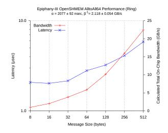
Fig. 9. Performance of the new (to version 1.3) contiguous all-to-all data exchange operation, shmem\_alltoall, for 16 processing elements
