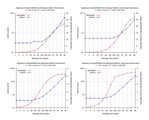
Fig. 4. Performance of non-blocking remote memory access routines.
