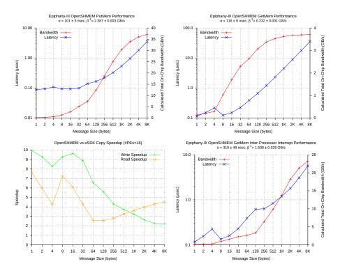
Fig. 3. Performance of optimized shmem\_put (top left) and shmem\_get (top right) for contiguous data exchange operations for 16 processing elements, speedup comparison with eLib (bottom left), and experimental inter-processor user interrupt for high-performance shmem\_get (bottom right).
