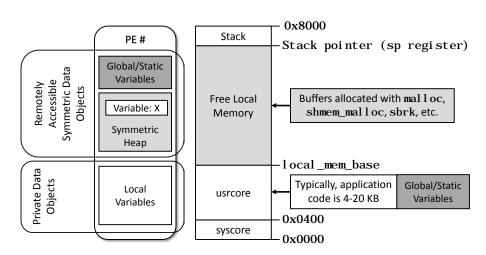
**Fig. 2.** The PGAS memory model (left) and the equivalent typical memory layout on an Epiphany-III core (right)
