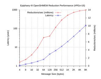
Fig. 8. Reduction performance for shmem\_int\_sum\_to\_all for all 16 processing elements. The latency and the number of collective reductions per second are shown. The effect of the minimum symmetric work array size for reductions, defined as SHMEM\_REDUCE\_MIN\_WRKDATA\_SIZE per the OpenSHMEM specification, is apparent for small reductions
