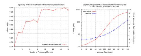
Fig. 6. Performance of shmem\_barrier for variable number of processing elements (left) and the performance of shmem\_broadcast64 for variable message sizes (right)
