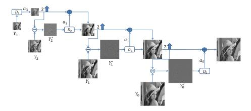
Fig. 2. First-pass of our method for a 4-layer cascade.  $\mathbf{Y}_0$  is the original image,  $\{\mathbf{Y}_3, ..., \mathbf{Y}_0\}$  denote each layer of the image  $\mathbf{Y}_3$  pyramid, and  $\{\mathbf{D}_3, ..., \mathbf{D}_0\}$  are the dictionaries.  $\mathbf{D}_3$  is learned from the downsampled image, remaining dictionaries are learned from the residuals  $\{\mathbf{Y}'_2, \mathbf{Y}'_1, \mathbf{Y}'_0\}$ .  $\alpha_n$  are the coefficients used to reconstruct each layer.
