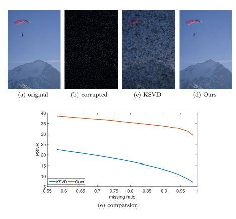
**Fig. 1.** (a) Original image. (b) Corrupt image where 93% the original pixels are removed. (c) Reconstruction result of KSVD, PSNR is 11.80 dB. (d) Reconstruction of our method, PSNR is 33.34 dB. (e) Reconstructed image quality vs. the rate of missing coefficients. Red: our method, blue: KSVD. As visible, our method is significantly superior to KSVD.
