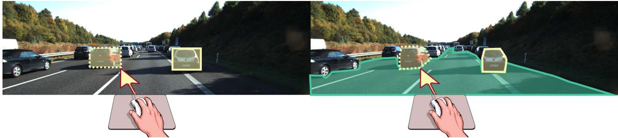
Figure 1: Ground truth obtained by human annotation: *left*) framing the rectangular bounding box (BB) of vehicle instances; *right*) delineating the contours (silhouettes) between the different classes of interest contained in the image, even at instance level.
