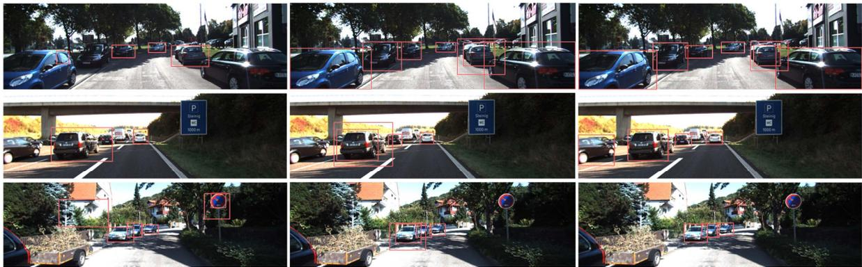
Figure 11: Vehicle detections when operating in the FPPI=1 regime. Left: DPM based on the SYNTHIA data considered in this chapter (SRC). Middle: Using the TAR0.1 version of KITTI-Det Train. Right: Adapting SRC by using TAR0.1 when applying SA-SSVM.
