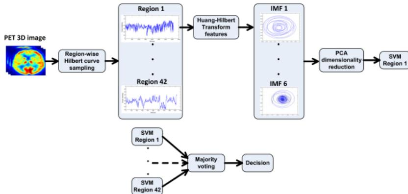
PET image classification using HHT-based features through fractal sampling
