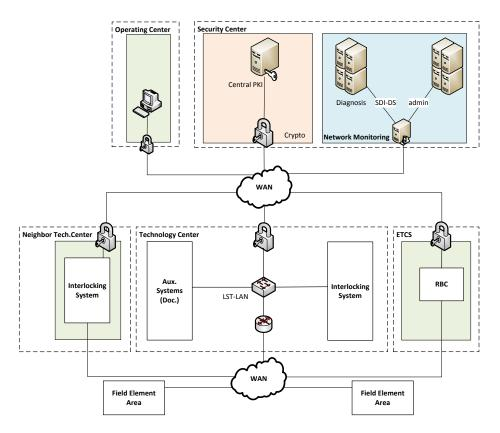
Fig. 1. Architecture of a typical signalling network.
