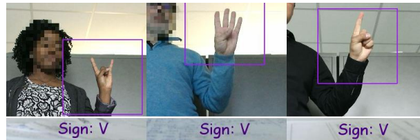
Fig. 6. Intended sign: “H”, recognised sign: “V” (left), intended sign: “4”, recognised sign: “V” (middle), intended sign: “D”, recognised sign: “V” (right)
