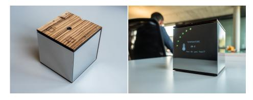
**Fig. 2.** ComfortBox is an interactive research tool designed to facilitate data collection in lab and in-situ comfort studies. The physical design is intended to help blend into the desktop setting and stay in the periphery of attention when not used.
