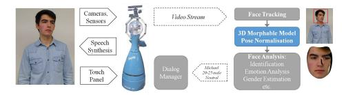
Fig. 7: Schematic overview of the framework for human-robot interaction on our SCITOS G5 platform. Our proposed landmark based 3D Morphable Model fitter acts as a pre-processing method for various face analysis tasks.
