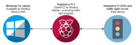
Fig. 2. Diagram of components in the SCADA testbed. Assembled using icon sets available at [16]
