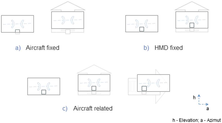
**Fig. 8.** Integration concept for the 360 degree top view inset in the HWD
