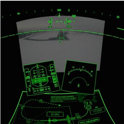
**Fig. 5.** Virtual aircraft-fixed cockpit instruments [19]
