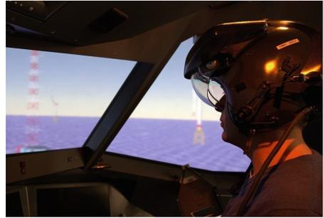
**Fig. 2.** See-through HWD in DLR's Generic Experimental Cockpit [4]
