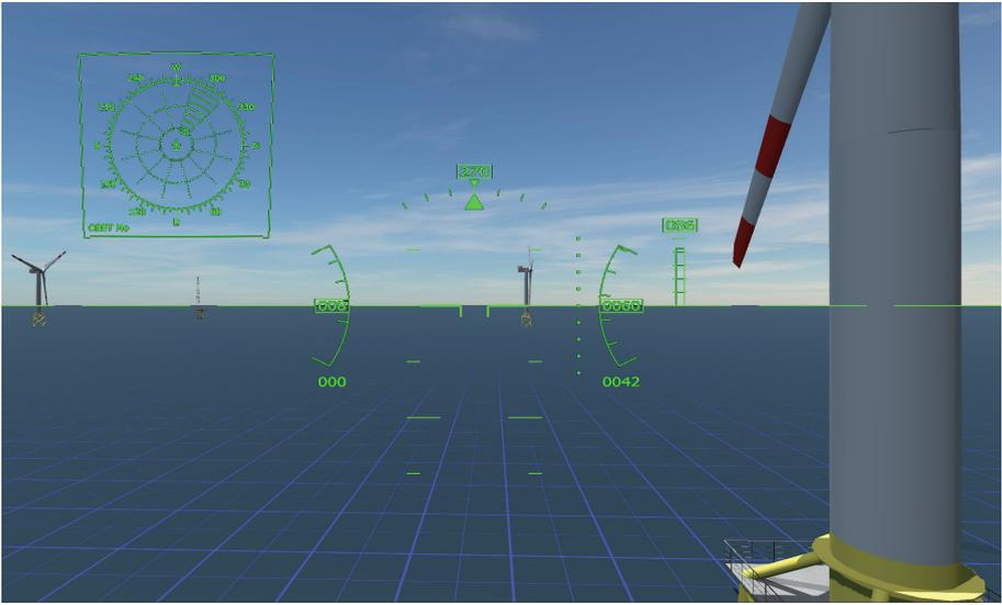
**Fig. 9.** HWD OAWS in case of conducting a hoist operation at the lower access point of an offshore wind turbine
