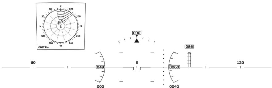
**Fig. 7.** Orthogonal coplanar 360 degree top view in a HWD depicting surrounding obstacles (Color figure online)
