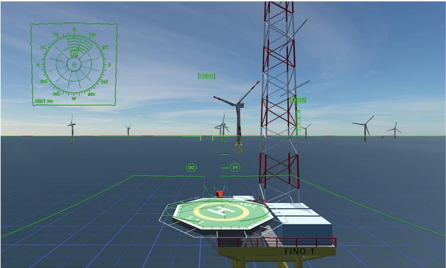
**Fig. 10.** HWD OAWS in case of landing on the research offshore platform FINO1
