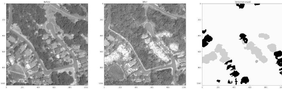
**Fig. 7.** Results of the change detection on the test subset of data in Santa Rosa without fine-tuning. Left: image taken before fires, center: image taken after fire, right: segmentation results black - non-damaged, gray - damaged buildings
