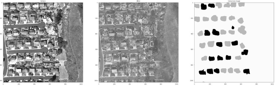
**Fig. 5.** Results of the change detection on the validation subset of data in Ventura. Left: image taken before fires, center: image taken after fire, right: segmentation results black - non-damaged, gray - damaged buildings
