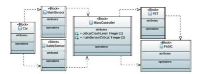
Fig. 3. bdd of the Airbag model
