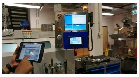
Fig. 3. Remote maintenance interface mounted on a HAAS control panel.
