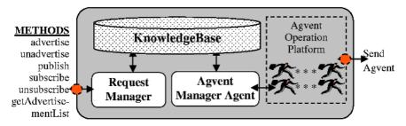
Fig. 2. Inner Structure of an Agvent Server
