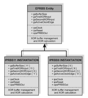
Fig. 3. Illustration of the template instantiation with the modified UML diagram
