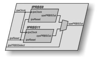
Fig. 2. Hardware structure of the presented example
