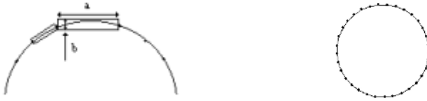
Fig. 1. a. Approximation using polygon segment b. Discretized boundary values of circle
