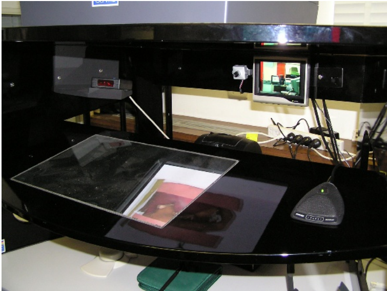
Fig. 3. Enhanced haptic workbench showing small CCD camera (top center), LCD monitor (top right of center) and microphone (right foreground).
