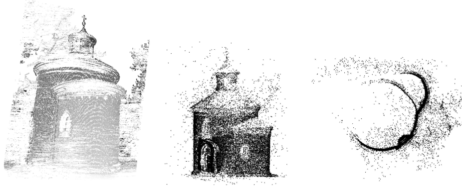
Fig. 4. The disparity map for the first two images in the second row in Fig. 2 and Point clouds for the St. Martin scene (a front and a top view). Only 2% of all points are shown
