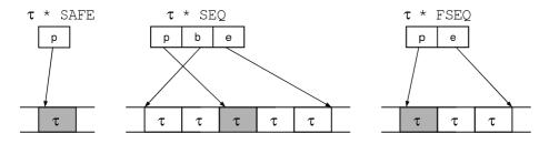
Fig. 1. SAFE, SEQ and FSEQ pointers, respectively, to the shaded memory locations
