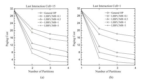
**Fig. 6.** Paging cost vs. number of partitions for the general OP scheme and the LIBP algorithm with different values of the call-to-mobility ratio, when (a) LI cell=15 and (b) LI cell=1
