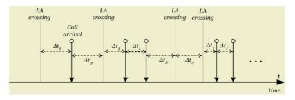
Fig. 3. Timing diagram of modeled user-network interactions during MT movement
