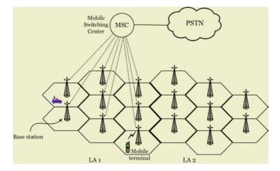
**Fig. 1.** Paging procedure in a mobile cellular network (the figure shown here is simplified, as other components involved with the paging procedure are omitted, such as the SS7 network and HLR/VLR databases. Additionally, the BSC/RNC is omitted, since its primary function is to maintain the radio resources of its base stations and is not directly involved in paging)
