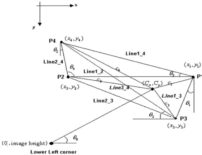
Fig. 4. The feature made from the extracted four points
