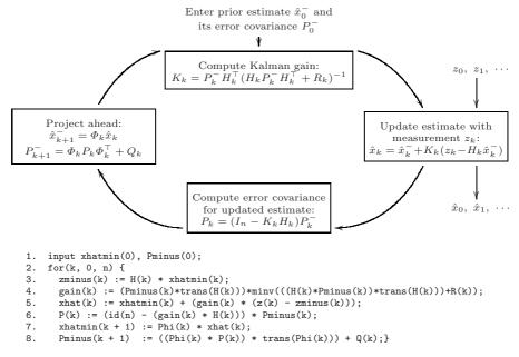
Fig. 1. Simple Kalman filter loop and intermediate code.
