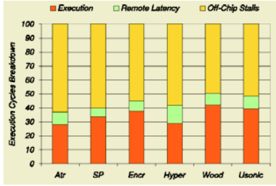
Fig. 4. Execution cycle breakdown for the default mode of execution.
