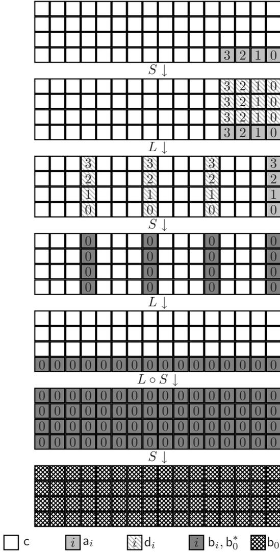
**Fig. 6.** The 3.5-round integral distinguisher for PRESENT. Top row of cipher block is word 0, bottom row is word 3. The rightmost column corresponds to the least significant bit (bit 0) in each word.
