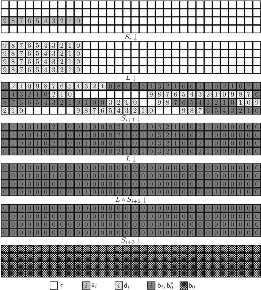
**Fig. 5.** The 3.5-round integral distinguisher for Serpent. Top row of cipher block is word 0, bottom row is word 3. The rightmost column corresponds to the least significant bit (bit 0) in each word.
