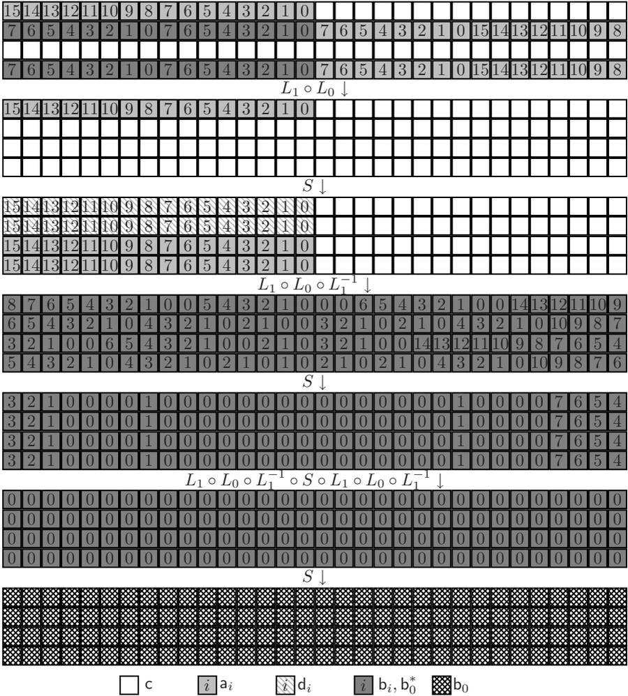
**Fig. 4.** The 3.5-round integral distinguisher for Noekeon. Top row of cipher block is word 0, bottom row is word 3. The rightmost column corresponds to the least significant bit (bit 0) in each word.
