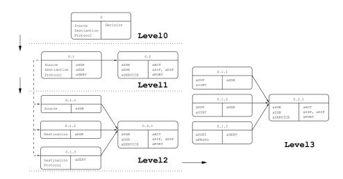
Fig. 1. The ARD diagram for the firewall.
