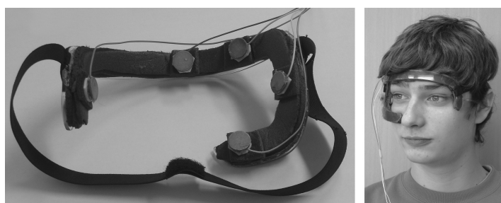
Fig. 1. Left: Five gold cup electrodes are integrated into the prototype of the EOG-Head Device, which is ergonomically designed for human heads. Right: A subject wearing the Head Device.
