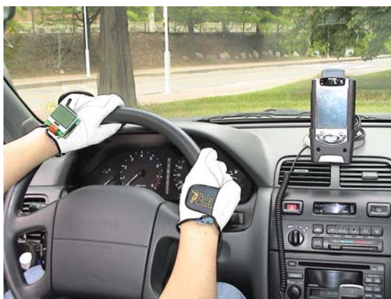
Fig. 2. Use of chording gloves in an in-vehicle infomatics and telematics environment
