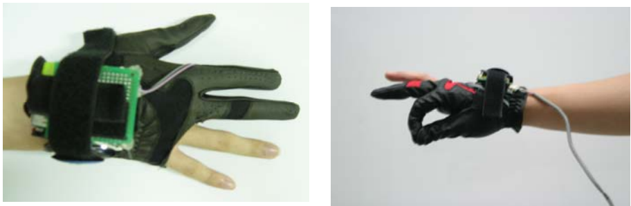
Fig. 1. The UbiHand Glove. The thumb acts as a ground to conduct electricity to the keys on the fingers made of silicon ink. It also contains an RFID reader so that it can sense and record what it touches or where it is.
