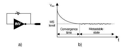
Fig. 1. Metastability employment scheme based on CMOS inverter a), and its convergence process b)
