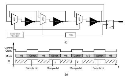
**Fig. 3.** Generic Meta-RO architecture a) and operational diagram b). The set of inverters could be used to form independent entropy sources (in metastable mode) or a regular ring oscillator to amplify and resolve the obtained random state.
