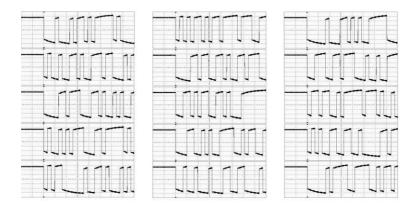
**Fig. 7.** Consequent runs of Meta-RO5st after restarting. Since after restarting, every generated sample is different, this is evidence that output of the proposed D-TRNG is not defined by a deterministic source.
