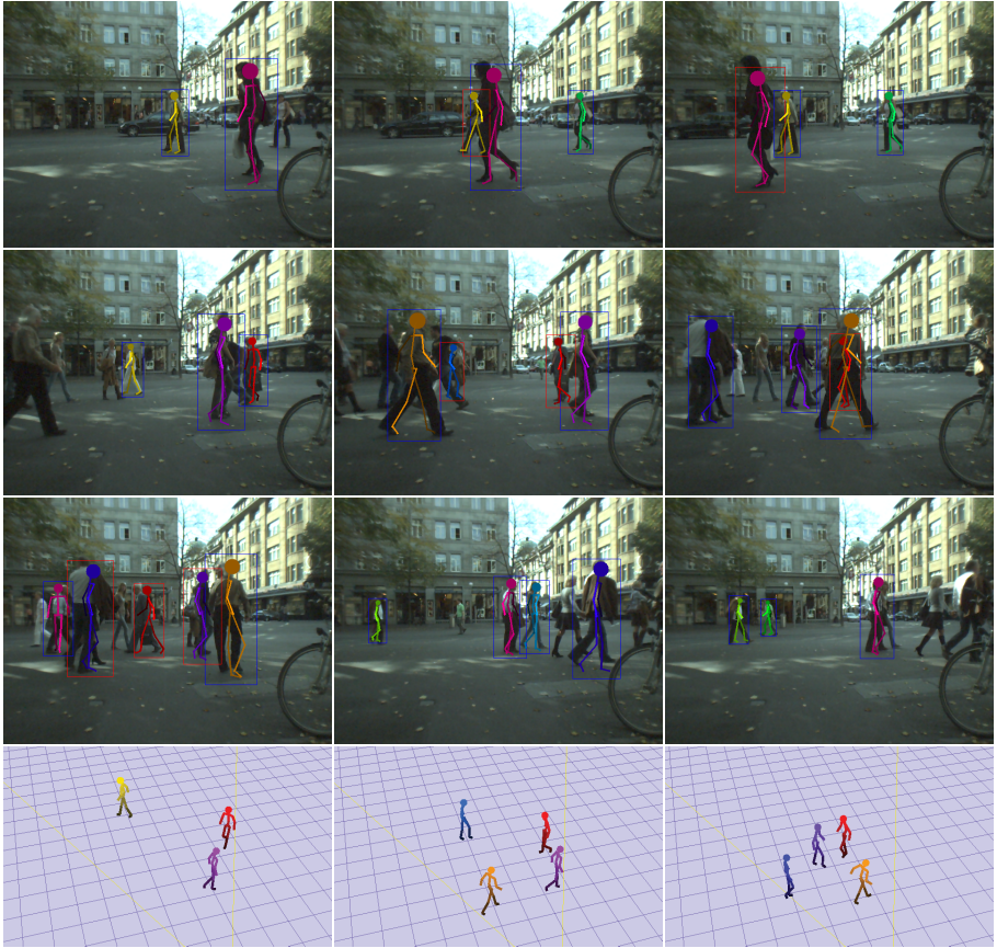
Fig. 5. Articulated multi-person tracking results for test sequence #1. The last row shows a 3D visualization of the estimated world state in the three images of the second row (This figure is best viewed in color).
