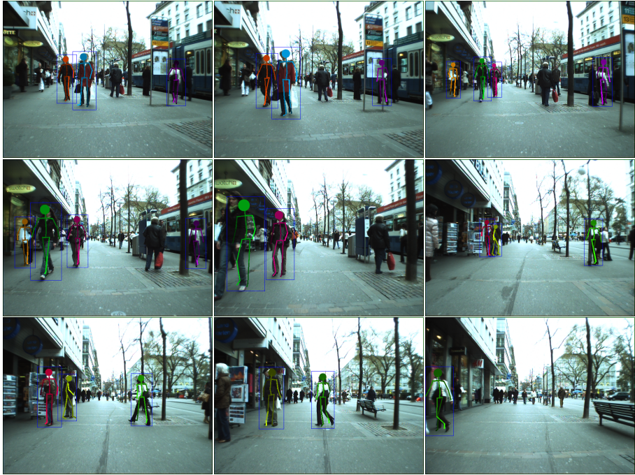
Fig. 6. Articulated tracking results for test sequence #2. Note the robust articulation estimates of tracked pedestrians under scale changes and egomotion. (This figure is best viewed in color).
