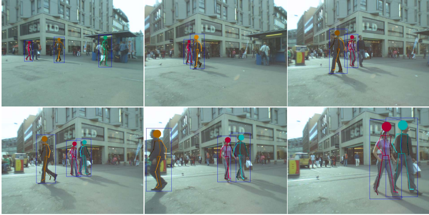
Fig. 1. An example for the articulated multi-person tracking scenarios considered in this paper. We address this task by first applying a robust multi-body tracker to handle the data association problem and identify individual tracks. An articulated tracker is then applied to each single-person track independently to infer precise body poses, which are in turn fed back to improve the observation model. As can be seen from our results, this procedure allows robust performance despite the presence of multiple people, temporary occlusions, scale changes, and camera motion.
