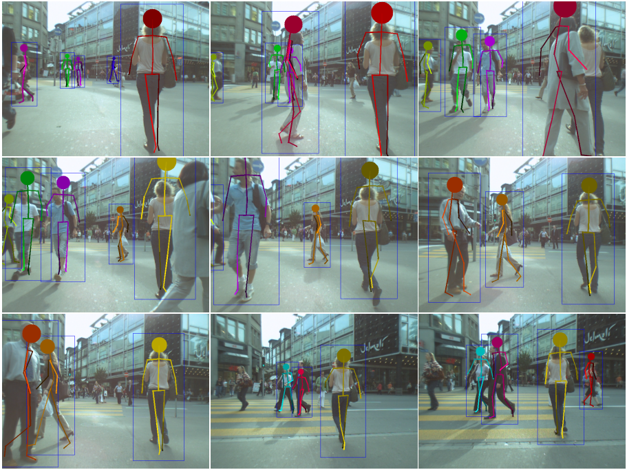
Fig. 7. Articulated tracking results for test sequence #3. This sequence shows a very challenging scenario with considerable egomotion and many pedestrians entering the visible scene at various distances and from different directions. (This figure is best viewed in color).
