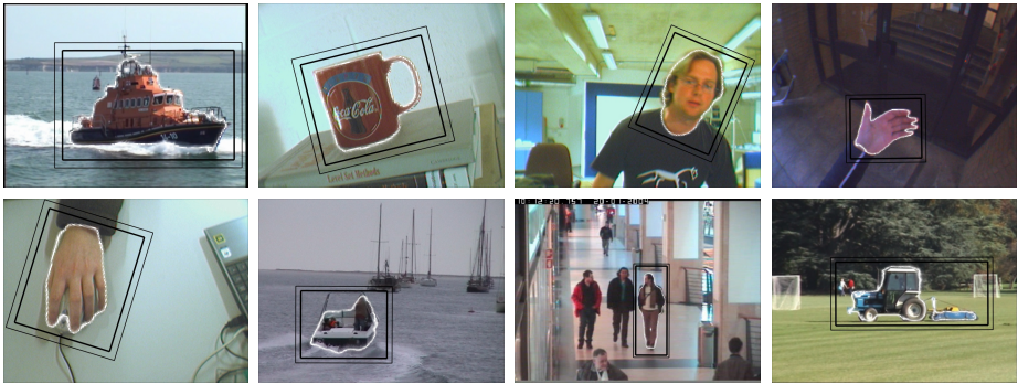
Fig. 3. A selection of video frames from the data sets: (1st row) lifeboat, Coca-Cola mug, a face and a hand filmed from a head mounted camera; (2nd row) a hand using a mouse, a speedboat, a person from the caviar data set [18] and a tractor. The white indicates the current segmentation and the two black boxes indicate the object coordinate frame.
