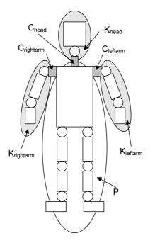
Fig. 4. Kinematically and dynamically steered joints in the conductor
