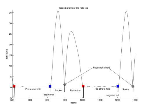
Fig. 2. Motion phases are detected from the speed profile
