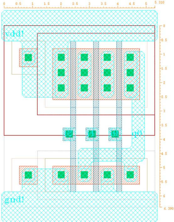
**Fig. 3.** Layout of the NOR-3 gate (UMC 0.18  $\mu\text{m}$ )
