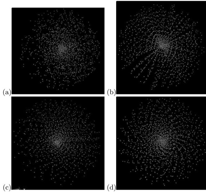
**Fig. 7.** Different sets of samples on  $SO(3)$  (a) 2000 random samples (b) 2048 Sukharev grid samples (c) 1944 icosahedral samples (d) 1944 HEALPix samples
