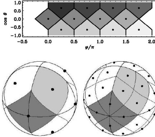
**Fig. 5.** Base grid of the HEALPIX sequence consists of 12 points. The cylindrical projection of the grid cells from  $S^2$  to  $(\cos(\theta), \phi)$  coordinates is shown. Each next resolution subdivides each of the spherical squares into 4 squares of equal area. Figures are borrowed from [7].
