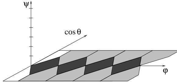
**Fig. 6.** The base grid of the proposed  $SO(3)$  sequence consists of 72 points. For the Hopf coordinates  $(\theta, \phi, \psi)$  the projections of the grid regions on each of the coordinates are shown. Grid regions for  $\psi$  are chosen according to the ordinary grid on  $S^1$ . The grid regions for  $(\cos(\theta), \phi)$  are obtained using the HEALPix method.
