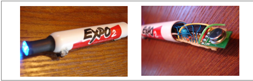
Fig. 2. Exterior view of current FireFly prototype with light emitting diode, power and momentary switches. CPU, power supply, and wireless communication components fit into a dry marker package and a user “draws” by pressing the momentary switch while moving the pen.
