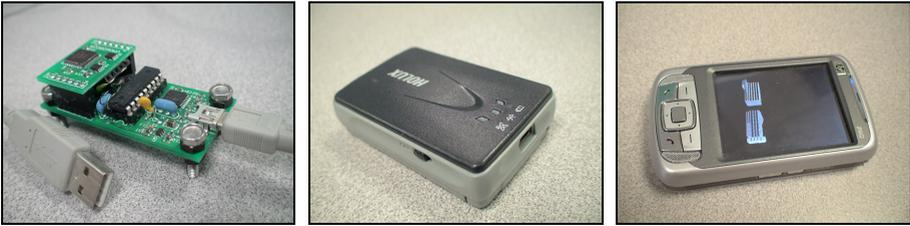
Fig. 4. The gyroscope, the GPS device and PDA
