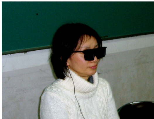
Fig. 2. An observer uses the specially designed glasses. The right and left liquid crystal shutters in the glasses alternately open and shut at a frequency of 30 Hz. If the observer is myopic and cannot see the LCD without glasses, he/she wears both the glasses for myopia correction and the glasses with liquid crystal shutters.
