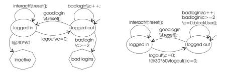
**Fig. 1.** (a) An automaton monitoring the bad logins occurring in a system; (b) The same automaton with recovery actions.
