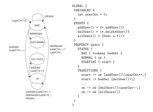
Fig. 2. The automaton and LARVA code of Example 2.
