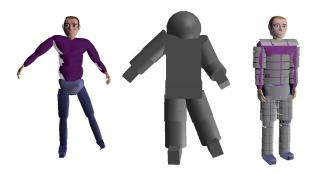
**Fig. 1.** Max's segmented body (left) with proximity geometries allowing for predicting touching of objects and identifying the touch receptor's corresponding limb (middle). Max's virtual body covered with over 200 virtual skin receptors (right).
