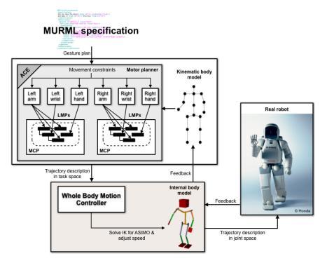
Fig. 4 Control architecture for robot gesture.
