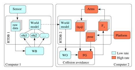
Fig. 4 Overview of the collision avoidance application: The *ARCADE* framework manages distributed computing and different update rates of the modules.
