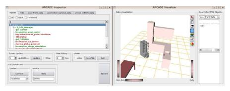
**Fig. 3** The *ARCADE* Inspector lists the tree of all database objects, provides access to the object data and a record functionality. The *ARCADE* Visualizer provides a 3D visualization of the current system state.
