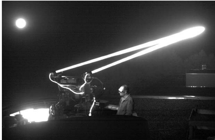
Fig. 11. Optical Ground Station Oberpfaffenhofen (OGS-OP) during the KIDO 2009 trials. Visible on the infrared picture is the beacon laser's backscatter due to haze.
